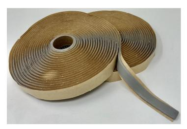
Foster® 14-40 HVAC Flange Tape is an extruded, pre-formed, double sided butyl tape furnished in rolls between silicone release liner. It is a non-hardening, solvent free, 100% solids sealant for sealing bolted flange joints in HVAC duct work. It bonds well to galvanized, aluminum, stainless steel and other metals forming an air tight gasket.
